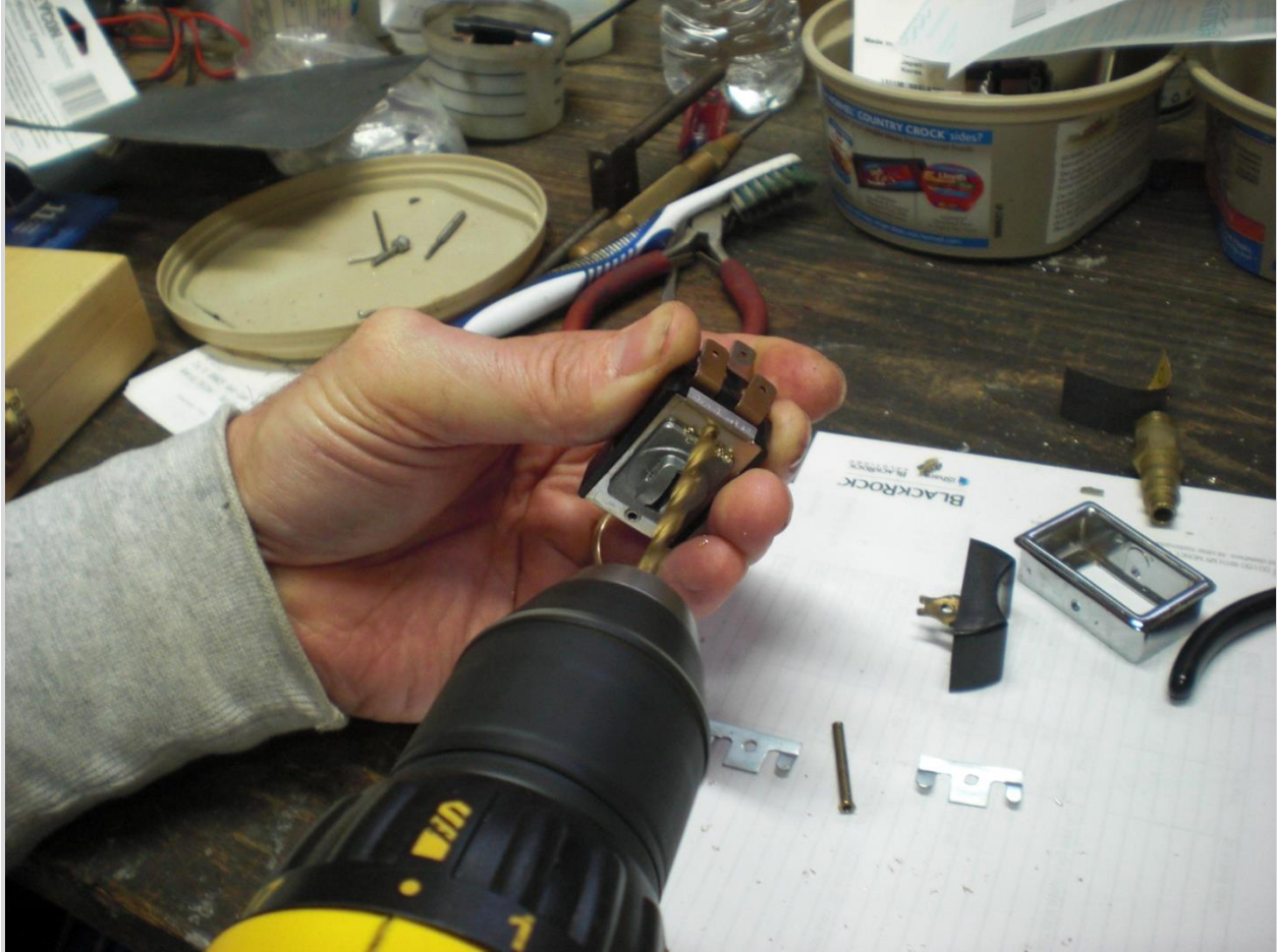
On this switch the two vertical rivets did not hold the bezel, only the base plate to the case.
