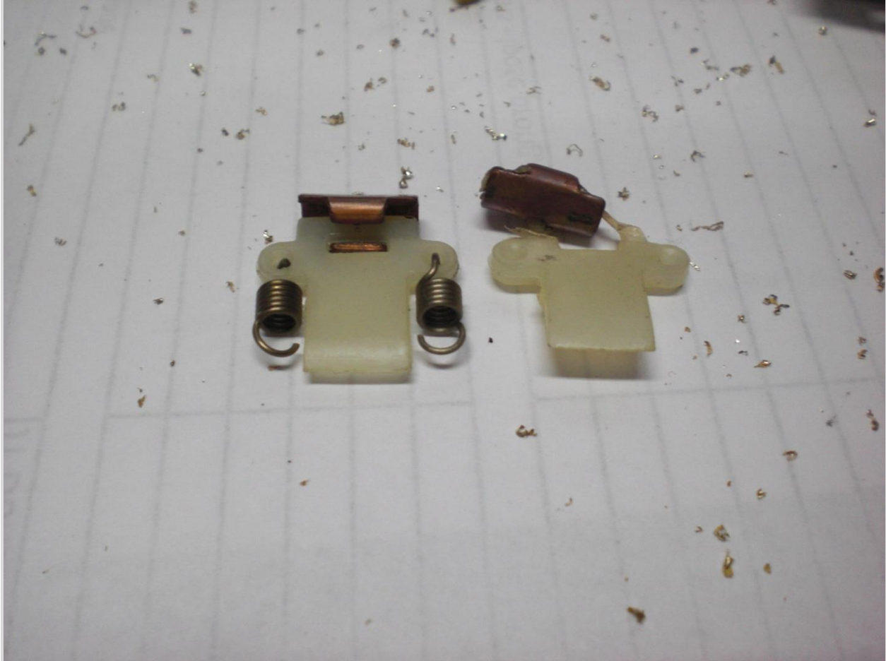
Note: The end of the spring that would attach to the base plate is open to the inside of the spade.
